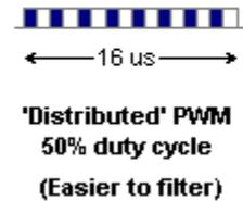
**The 'on/off' PWM duty cycle:** Starts with eight pulses 'high' for the first part of the PWM cycle, then finishes with eight 'low' pulses for the remainder of the PWM cycle. The ratio of the percent 'high' time to the percent 'low' time is called the duty cycle. Note that the PWM frequency of the 'on/off' PWM for any duty cycle in the drawing above is:  $F = 1/P = 1 / 16\mu s = 62.5\text{KHz}$ .
