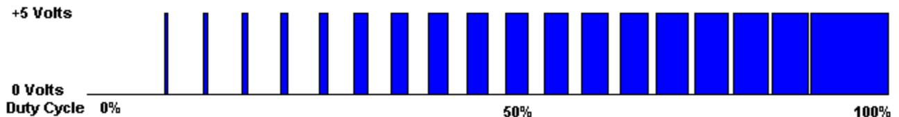
**Uses for PWM:** 1) To digitally create an analog output voltage level for control functions and power supplies.
