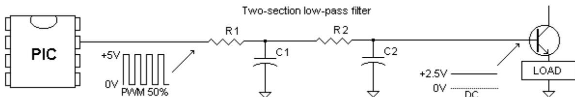
The above figure shows a PIC microcontroller generating a 50% duty cycle PWM signal at 5,000 Hz, a two-section 5,000 Hz low-pass filter and a pass-transistor with a direct current input of +2.5 Volts. The filter frequency =  $1/2 \pi RC$  for each section.
